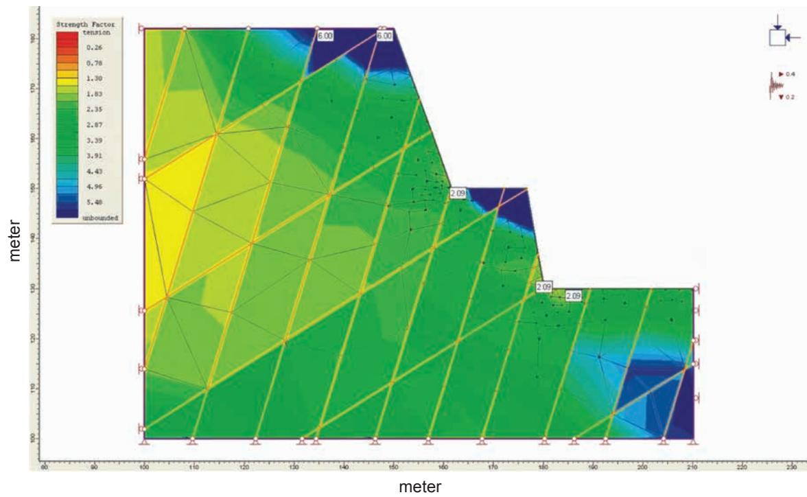
Figure 9. Simulation model of safety factor in dynamic condition at line A-A'
