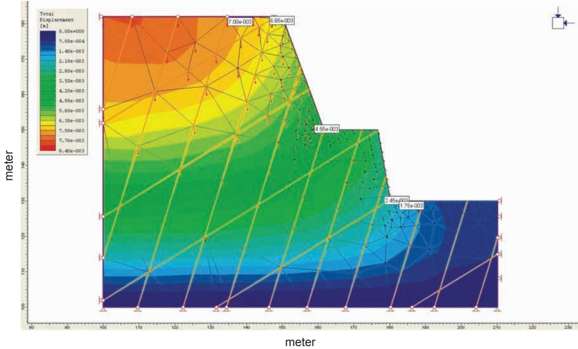
Figure 6. Simulation model of displacement distribution in static condition at line A-A'
