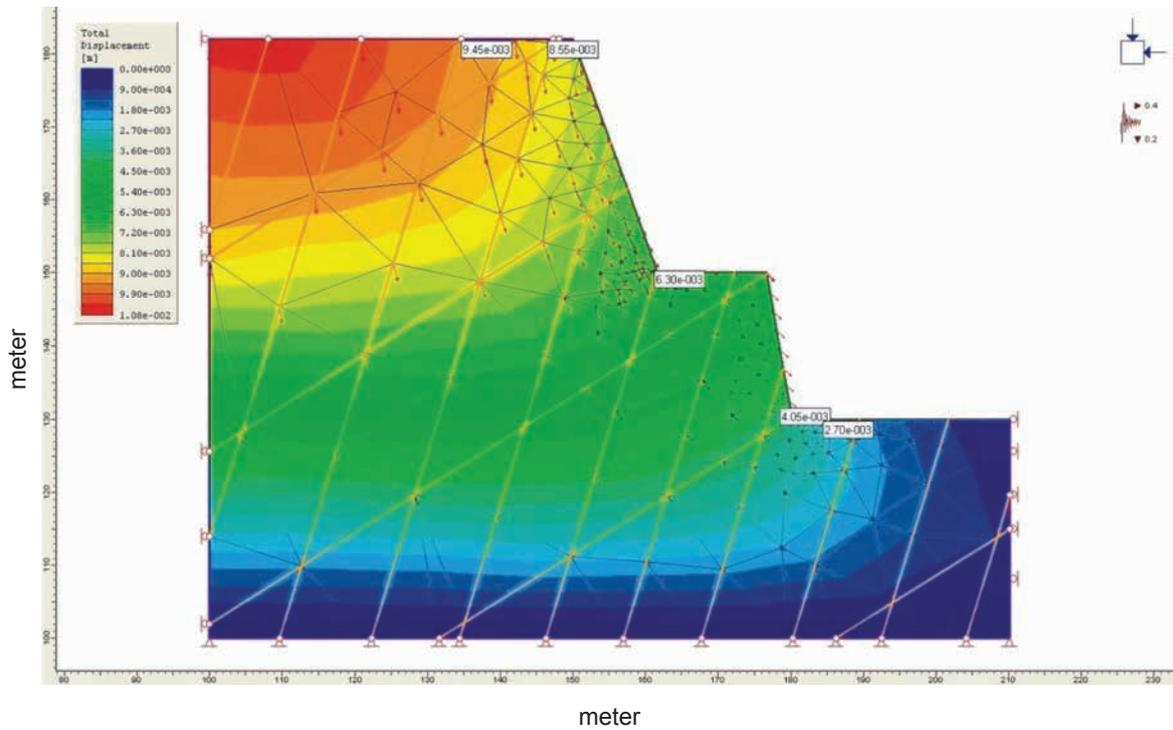
Figure 7. Simulation model of displacement distribution in static condition at line A-A'
