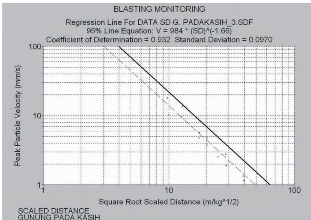
Figure 5. Graph of correlation between PPV and scaled distance (Basuki, 2011)
