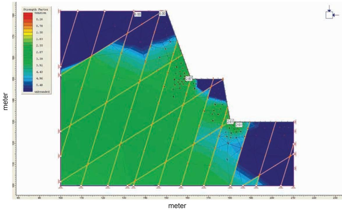
Figure 8. Simulation model of safety factor in static condition at line A-A'
