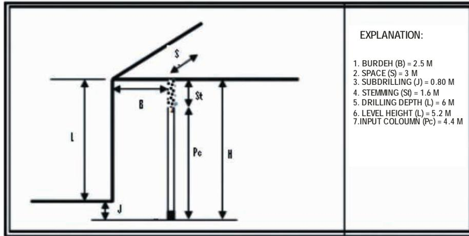
Figure 3. Blasting geometry
