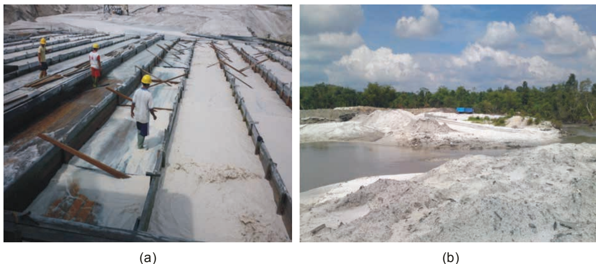
Figure 5. Sluice box for concentrating tin-bearing minerals at PT Koba Tin-Indonesia (a) and tailing sand from tin processing that contains REE-bearing minerals (b). The REE-bearing minerals are commonly monazite, xenotime and zircon (Wahyudi et al. 2009)
