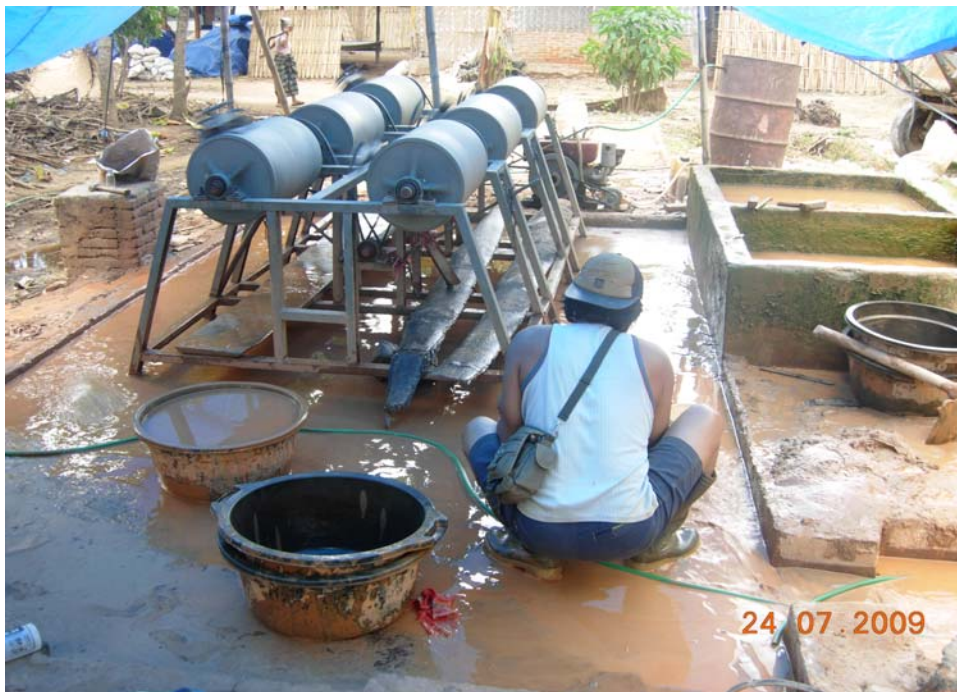
Enclosure C. Gold amalgamation mill in Lombok island (Yunianto, et al. , 2009)
