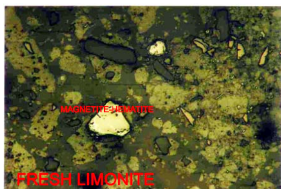
Figure 4. Microscopical observation of fresh Pomalaa ore
