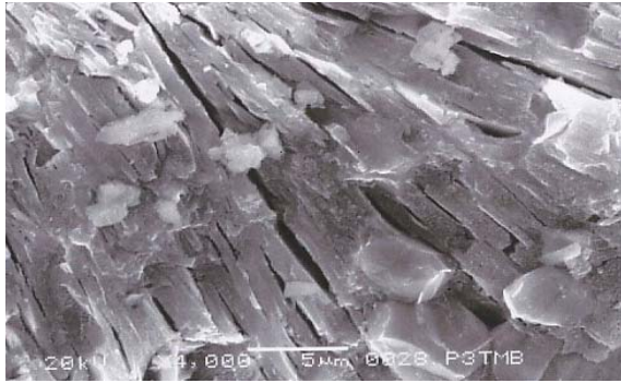
Figure 5b. A micrograph texture of the composite of reference castable refractory (CAJ-16)
