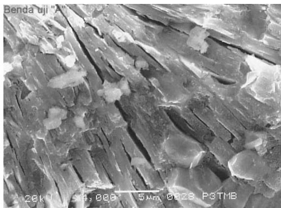
Figure 8d. Micrograph texture of the composite of reference castable refractory (CAJ-16), regular-lengthwise
