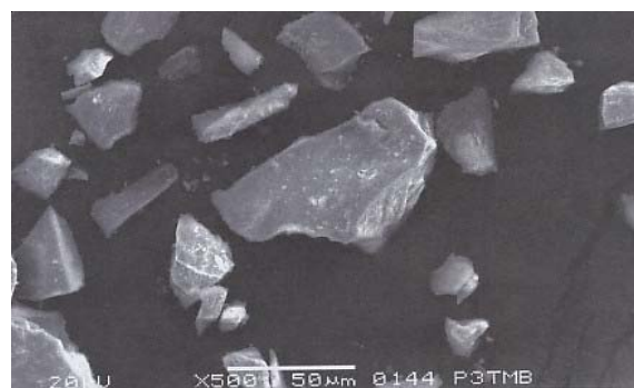
Figure 6c. Micrograph texture of fly ash burning at 1350°C, 0.5 hours, magnify 3000x, after crushing/grinding
