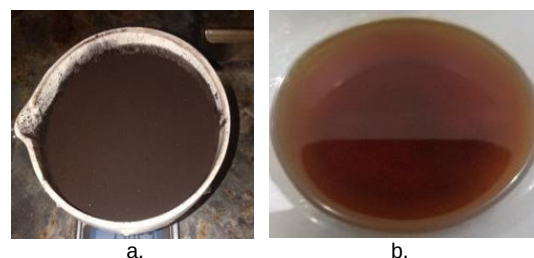
Figure 1. Lignite (a) and heavy oil from catalytic cracking of Polypropylene-Low Density Polyethylene plastic waste pyrolysis oil (b)
