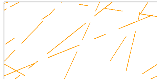
Figure 3. Joint network model with random joint length, orientation, and persistence
