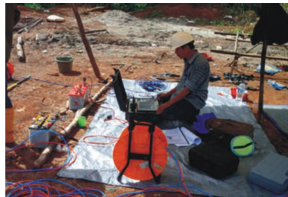
Figure 1. Downhole seismic measurements in a borehole
