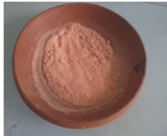
Figure 5. A photo of cerium oxide sample as raw material for reduction experiment
