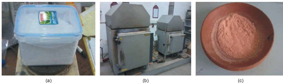
Figure 2. Photos of (a) cerium oxalate samples; (b) Muffle furnace for calcination process; (c) cerium oxide as calcination product
