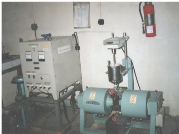
Figure 2. Magnetic ferro filter instrument
