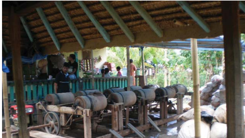
Figure 6. The processing of gold by using ball-mill at Sekotong, West Lombok
