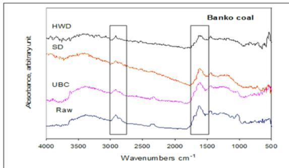
Figure 6. FTIR spectra for the raw and upgraded coals
