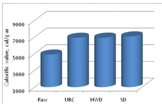
Figure 5. Calorific value of the raw and upgraded coals
