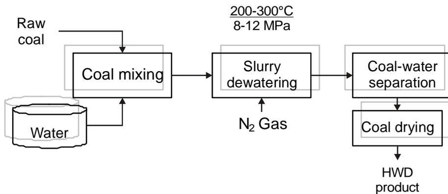
Figure 3. Block diagram of hot water drying process
