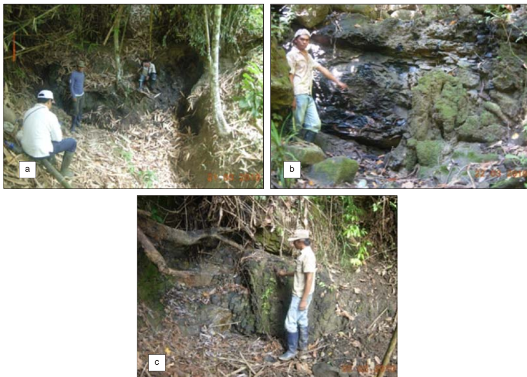
Figure 3. The coal deposits in the studied area, mostly dominated by the bright coal a. Seam A (1.5 m), dipping 23° to northeast b. Seam B (4.0 m), dipping 28° to northeast c. Seam C (1.5 m), dipping 25° to northeast
