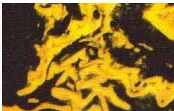
**Figure 6a. Suberinite showing broken-cell structure (yellow),  $R_{vmax}=0.37\%$ , brown coal. Field width 0.23 mm, fluorescence mode.**
