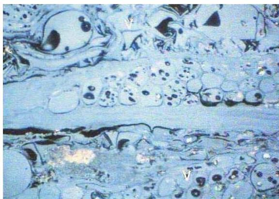
**Figure 5. Vitrinite with well-preserved cellular structure.  $R_{vmax}=0.36\%$ , brown coal. Field width 0.36 mm, reflected white light**
