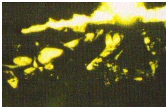
**Figure 7a. Exsudatinite (yellow),  $R_{vmax}=0.34\%$  (brown coal). Field width 0.42 mm, fluorescence mode.**
