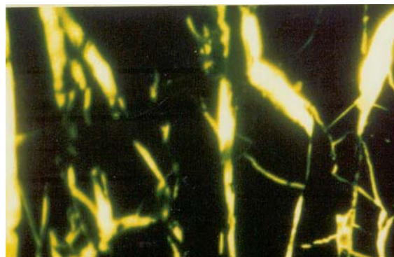
Figure 11. Exsudatinite (yellow) infilling the fractures of vitrinite (black). Rvmax: 0.65 %, field width: 0.28 mm, fluorescence mode
