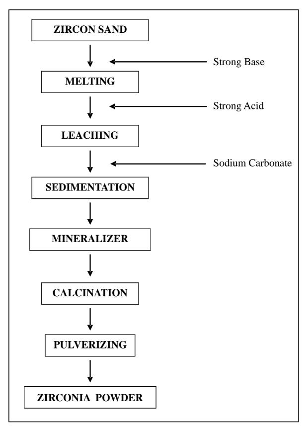
Figure 3. Flow chart of making zirconia powder
