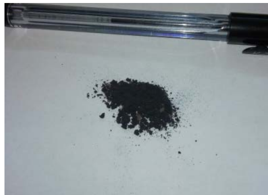
Figure 9. Calcined manganese carbonate
