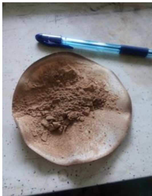
Figure 8. Precipitated manganese carbonate
