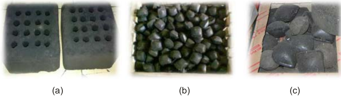
Gambar 4. Briket batubara : (a) sarang tawon (BKG); (b) telur (BPG); (c) briket Palimanan (Titan)
